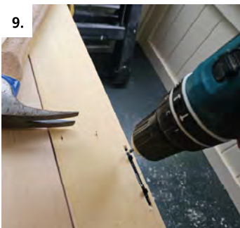
Screw each connector into place (both screws at same time to keep alignment centered)
