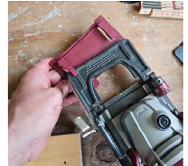
Set biscuit joiner to "20" and use spacer plates or stop square to achieve desired slot height
