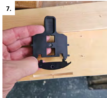
Place clamex S-20 connector onto alignment/insertion tool
