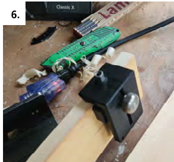
Drill 6mm holes for male connector halves using alignment tool or drill jig
